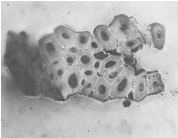
FIG. 6—A cross section of a jute fiber ( \times 40 ).
